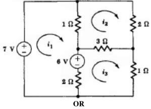
2 Find the current delivered by the source for the circuit shown in figure.
